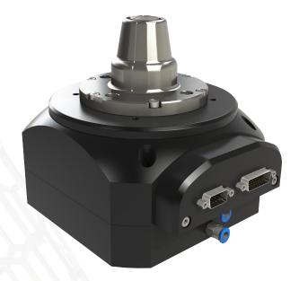
The RTS-150-3C is a high-precision rotary motion system with integrated 3C work holding. Designed specifically laser tube processing, it offers excellent angular accuracy, runout, wobble, and smooth low-speed profiling. It's low-friction pneumatic drawbar design enables precise clamping force adjustment. For more specific details on the base stage, please see the datasheet for the RTS-DD-150-BB-(C/D/E)-A-S-0-00. Contact Griffin Motion for further details on the product, pricing or lead time.
