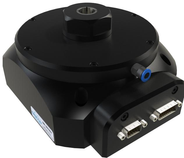
The RCS-150 is a high-precision rotary stage designed for demanding laser tube processing applications. It features an integrated ER25 collet system that provides automatic gripping with adjustable clamping force to accommodate a wide range of materials and wall thicknesses. Its direct-drive rotary architecture delivers smooth motion, excellent accuracy, and zero-backlash performance. Contact us to learn how the RCS-150 can enhance your laser cutting or welding system.
